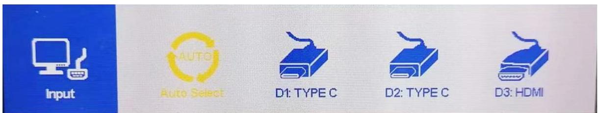
Press **EXIT** key to bring up the Input , press the</> key to select the signal input, press **Exit** key to exit
